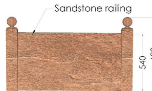
1 Red Sandstone Railing acting as a physical barrier in between the arched openings of the bays to maintain a proper circulation for the visitors
